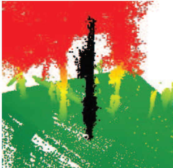
Figure 2.10: Result of a Min-Cut Based Segmentation. Black pixels represent the foreground cluster (a street light). Retrieved from Golovinskiy et al. [26].
