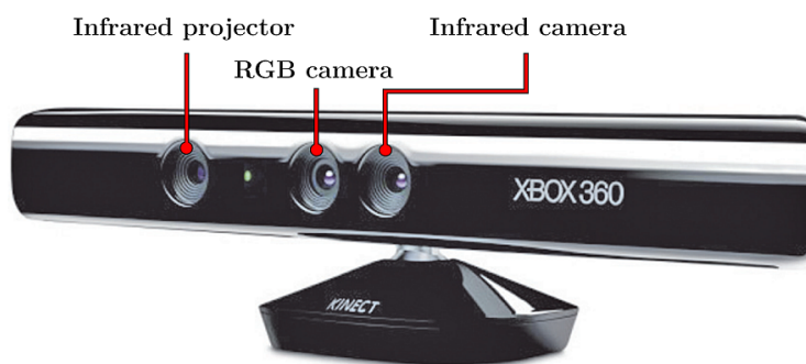
Figure 2.1: The Microsoft Kinect and its main components. Modified after Zhang [85].
