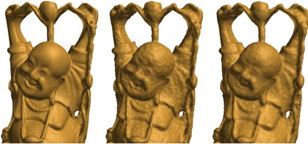
Figure 7.4: Left: input model buddha (noise: 0.0034, see Table 7.1). Middle: reconstruction with reference APSS [GG07] (reference implementation with marching cubes). Right: local reconstruction (positions+normals) with our method and Screened Poisson [KH13] to generate the mesh.
