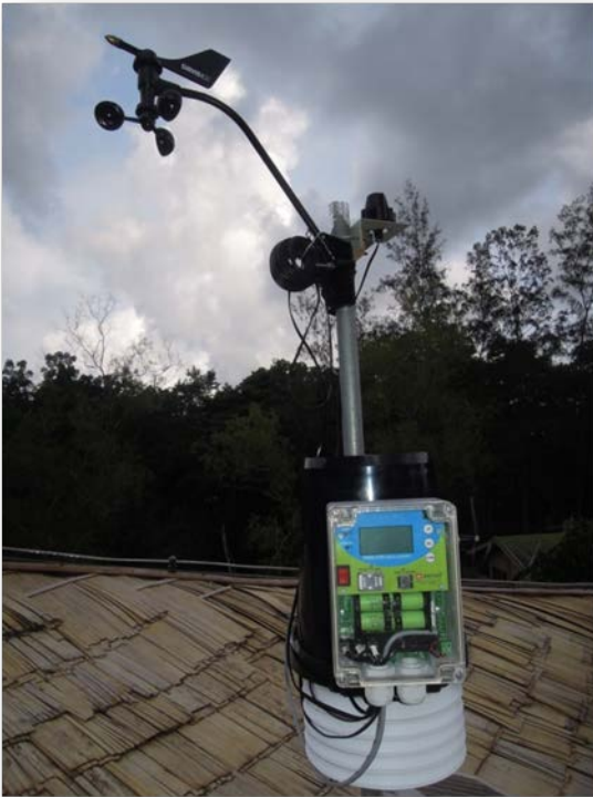
Figure 11: Weather station on the roof of the building
