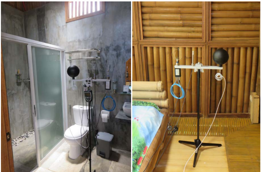
Figure 18: Test set-up in the bathroom and in the bedroom
