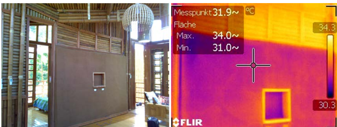
Figure 9: Centre wall as thermal mass; thermographic photo showing lower peak temperatures
