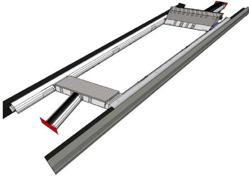
Figure 13. 3D model of the Schottenring metro station
