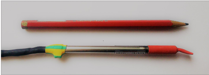
Figure 4.1: Photograph of the small neutron detector used for time-dependent measurements. Size comparison with a standard pencil. Both end parts are isolated with heat shrink tube. The bulge in the left end is produced by a clamp used to connect the outer wire of the coaxial cable with the detector tubing, a bad connection suspected to be the cause of a problematic blind count rate, as mentioned later on.
