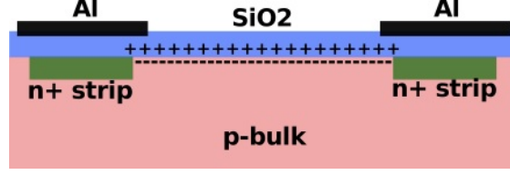
Figure 4.7: Schematic drawing of the accumulation layer for the opposite-sign oxide- and bulk-charge case.
