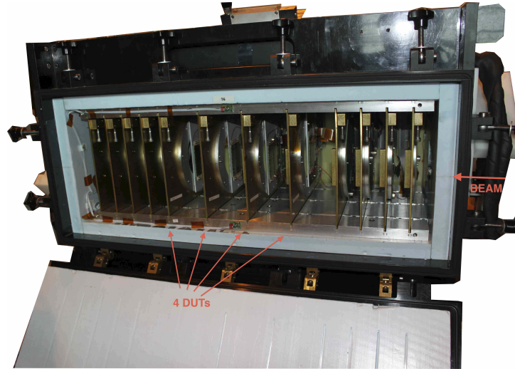
Figure 7.4: Picture of the Silicon Beam Telescope at the H4 beam line at the SPS North Area at CERN. The first and last four slots are occupied by the reference detectors. The picture shows the new cooling box that can hold up the four detectors under test (DUTs).
