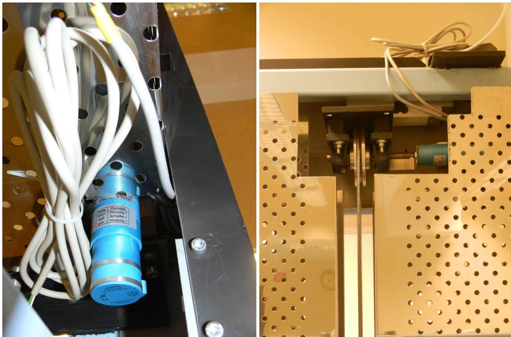
(b) Attached force (load cell) and way (rotary encoder) sensors.
