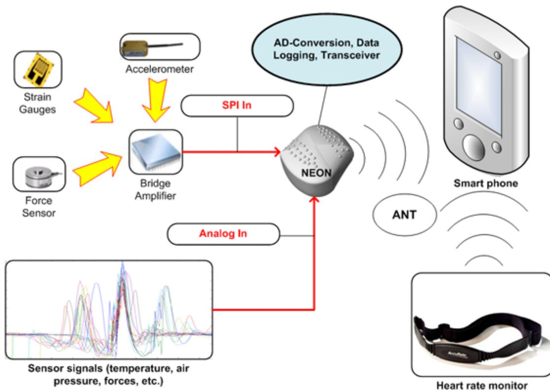
Figure 4.3: Integration of the NEON sensor platform in the mobile coaching concept.
