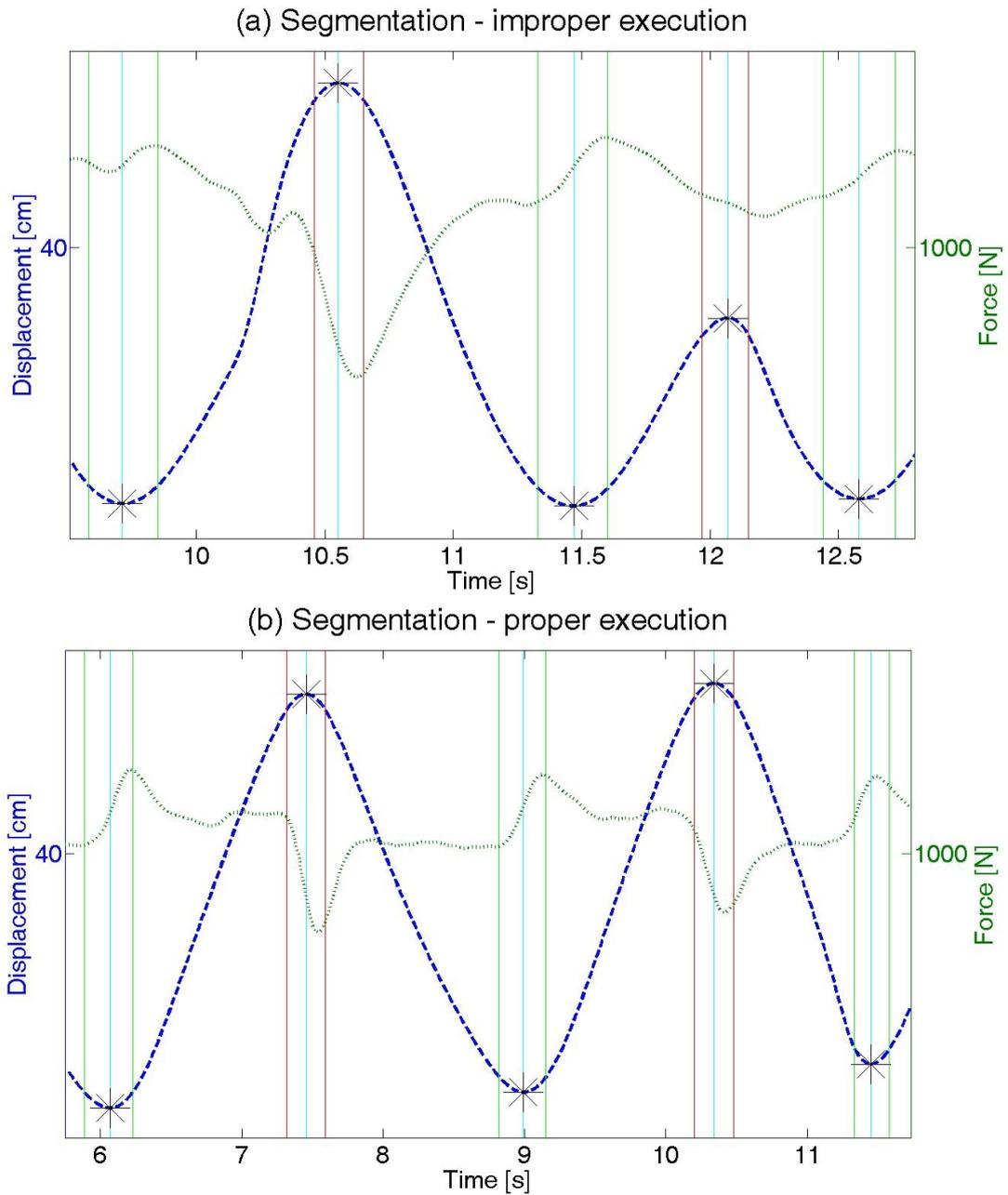
Figure 7.7: Illustration of the segmentation process for an improper (a) and proper (b) execution applied on the same data as in Figure 7.4. The displacement data was segmented into single repetitions based on peak detection techniques (marked by asterisk). The red and green lines indicate the starting and ending points in time of the holding phases after the concentric and eccentric actions.
