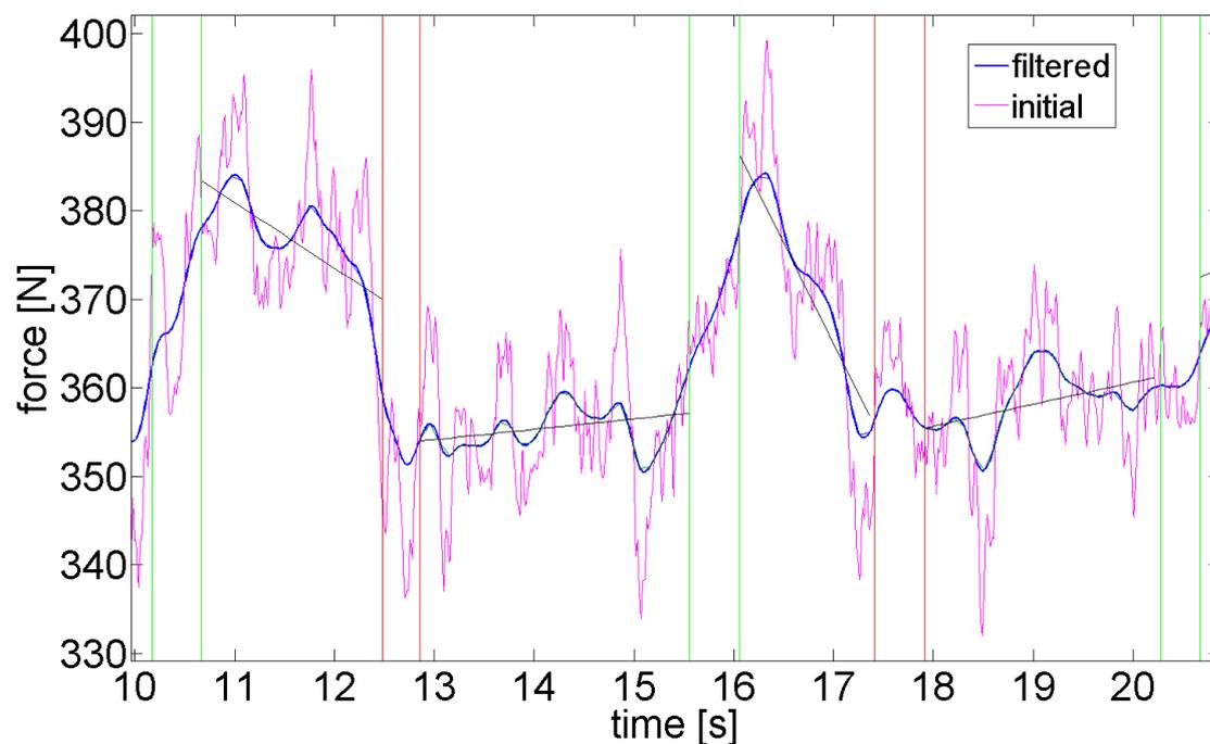
Figure 7.8: Segmentation of the force data into two repetitions and exemplary feature visualization (regression line).
