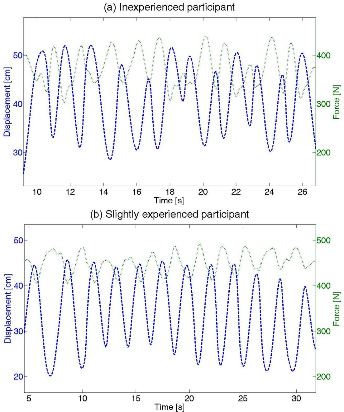
Figure 7.5: Comparison of the recorded time series of an inexperienced (a) and a slightly experienced (b) female participant with similar biographical characteristics using the same load.
