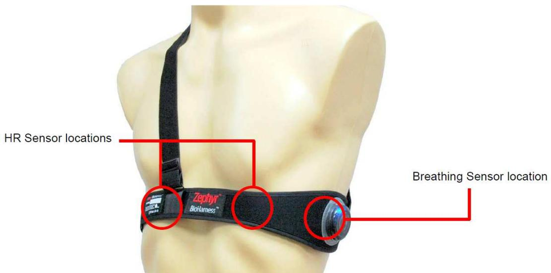
Figure 8.3: Appearance of the BioHarness chest strap with sensor locations (with permission from Zephyr, 2013b).
