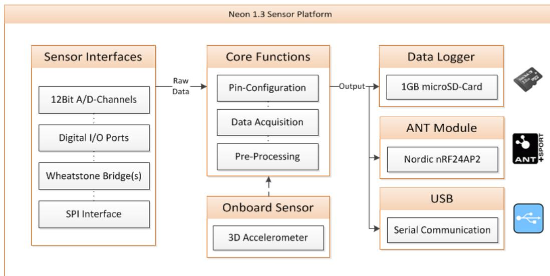
Figure 4.2: NEON sensor platform with integrated ANT chip.
