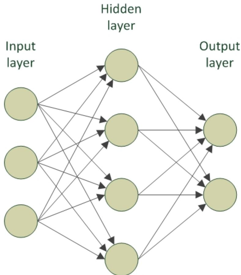
Figure 7.6: The typical design of an ANN with input, hidden and output layers, respectively consisting of three, four and two neurons.
