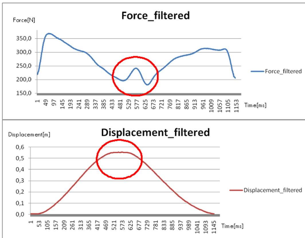
Figure 7.1: Filtered cable force and weight displacement data of an execution by an inexperienced individual on a sensor-equipped incline bench press machine collected at 200 Hertz (Hz) with a load of 30 kilograms (kg). The red circles label the turning point of the repetition, indicating the discrepancy of the measured channels with appearing force fluctuations.
