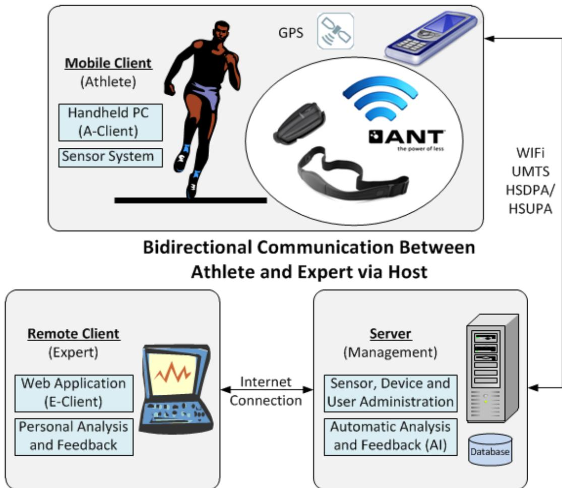
Figure 2.1: Overall concept of the system (bidirectional approach).
