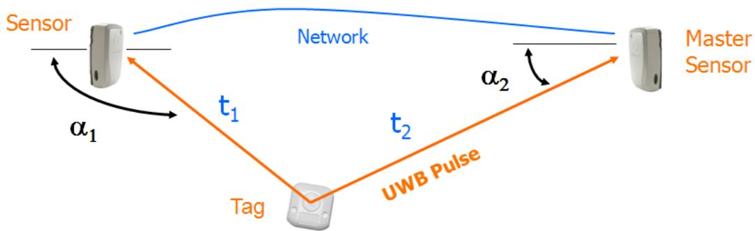
Figure 3.2: Position detection principle on the basis of gathered parameters like TDA and AOA (with permission from Ubisense, 2013).
