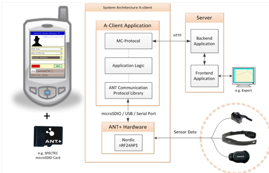
Figure 4.6: Communication between A- and E-Client.
