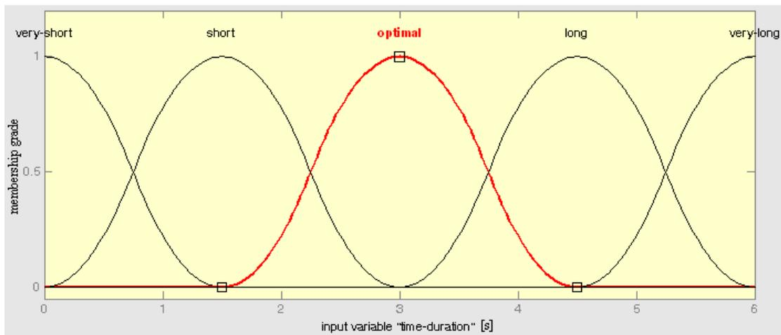
Figure 7.13: Exemplary fuzzy sets for the input variable mapping the time duration to a value between 0 (improper) and 1 (proper).
