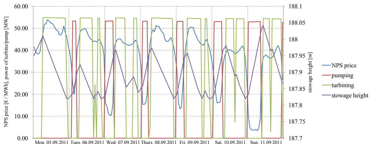
Figure 6.10 Operation plan of the PST-HPL Kymmen during one week in September 2011. The left y-axis actually has two axes overlapping - one for the NPS price and one for the power of the turbines/pumps. The right y-axis indicates the values of the stowage height.
