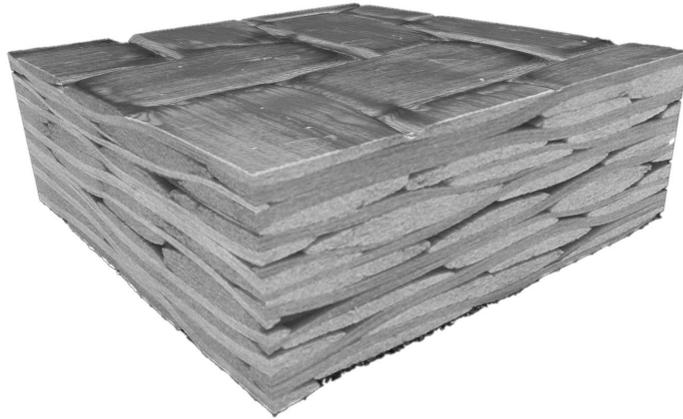
**Figure 2.5:** Rendering of a CT scan of a 2/2 Twill weave carbon/epoxy textile. Some of the unreinforced matrix pocket material is removed using segmentation tools for the sake of clarity.
