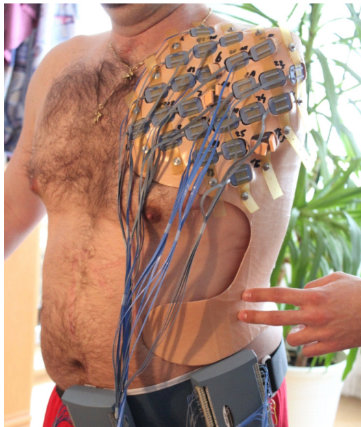
Figure 2.7: Fourth approach of the electrode array build-up, using a patient specific socket with all electrodes incorporated.
