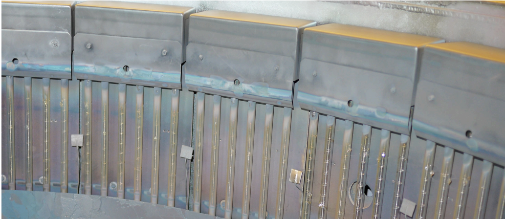
Figure 4.1: MP: Heaters 8 to 12 and Thermocouples TH8.5 to TH11.5. In heater 11 the hole in the middle through which pyrometer 11 detects the radiation from outside is visible.
