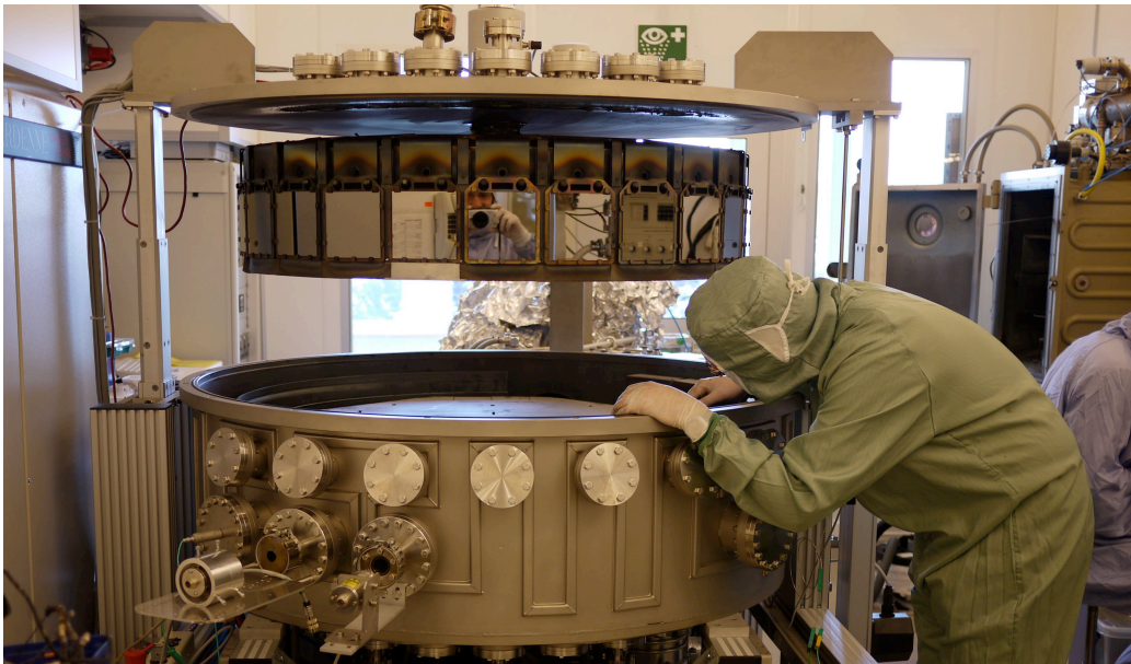
Figure 3.3: The MP vacuum chamber with open lid.
