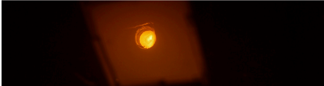
Figure 3.2: Liquid Al source heated by the electron beam
