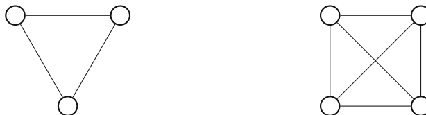
Figure 2.1: Left: a complete graph with three vertices ( K_3 ), called a triangle or a cycle of length 3 ( C_3 ); Right: a complete graph with four vertices ( K_4 )
