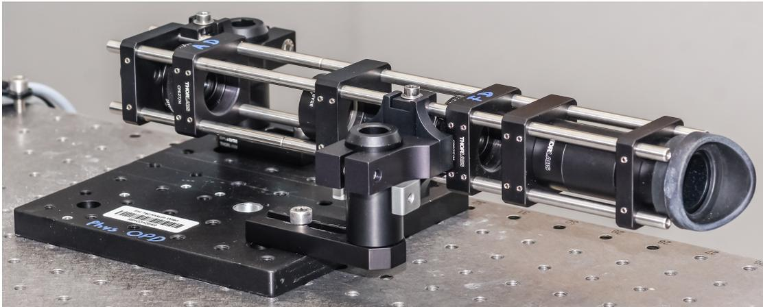
Figure 4.19: The breadboard with the projection optics is mechanically compatible to the breadboard of the [MTE](#)-setup. They can easily be exchanged by two mounting screws.
