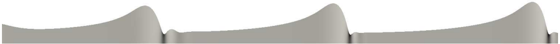
Figure 4.2.: Exemplary result of an isothermal ALE-simulation with interTrackFoam from OpenFOAM. Crosswise coordinate is scaled by 5, the grayscale indicates the pressure P . The parameters are different from the ones in Figure 4.1.
