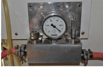
Figure 2.8.: Control valves for Helium gas flow. The screw on the left hand side is used for coarse justification and for fully opening the valve. The micrometer screw on the right hand side is used for fine adjustments, while the left one has to be fully closed. The gauge can be used for roughly tuning the pressure inside the VTI. For more exact values use the barometer (see 2.1.5)
