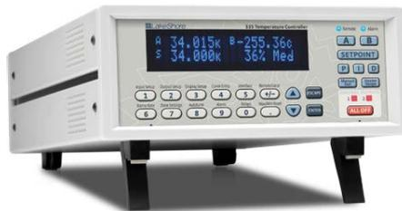
Figure 2.3.: LS Model 335 temperature controller
