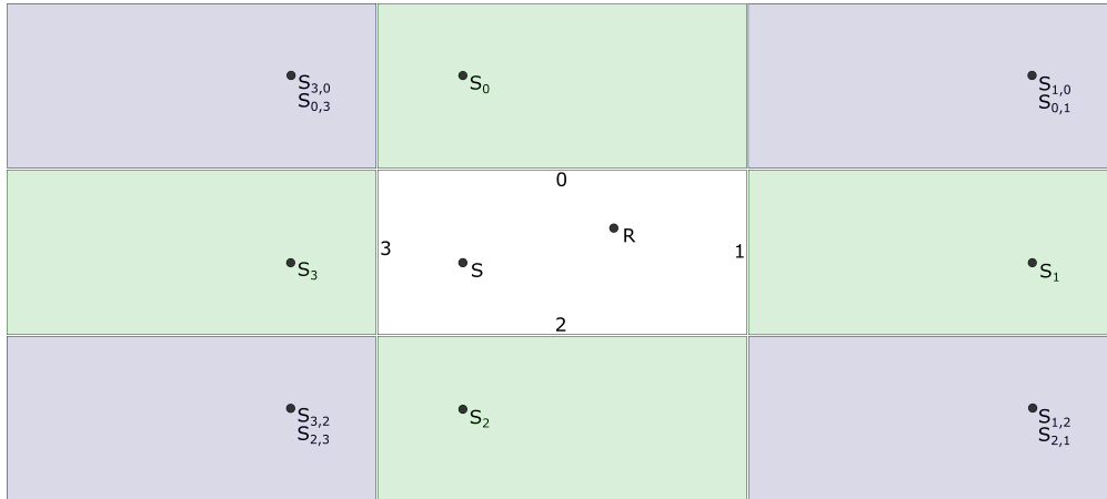
Figure 2.5: Calculation of image sources. S_x : image sources of first order; S_{x,y} : image sources of second order.
