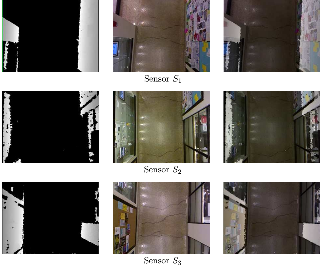
Figure 2.3: Kinect sensor field of view; raw depth data stream (left), RGB stream (middle) and both data streams in an overlay (right).
