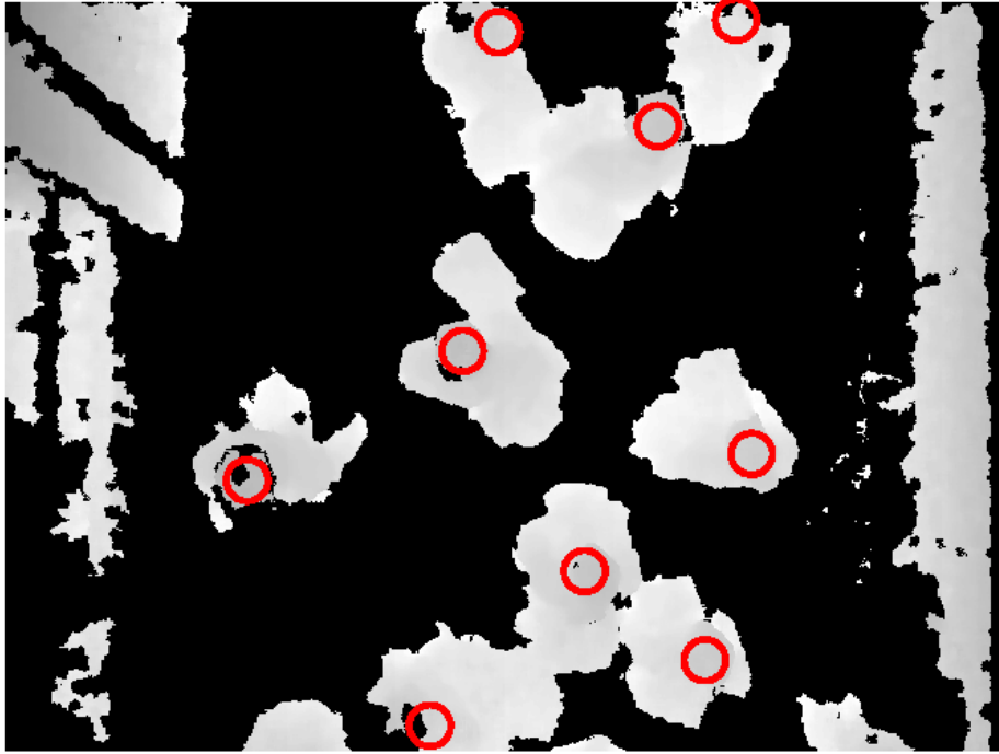
Figure 2.7: Kinect depth raw data in 3D (gray) with manually annotated head positions of individuals (red circles).
