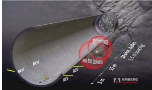
Figure 1.2.: TSP: Measurement layout of the 3D Tunnel Seismic Prediction method consisting of usually 4 receivers (RCV) and 24 shot points. (Dickmann and Krueger, 2014)
