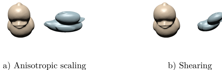
Figure 3.3: Affine transformation. Figure a) is only transformed by an anisotropic scaling and Figure b) by shearing along the z axis.
