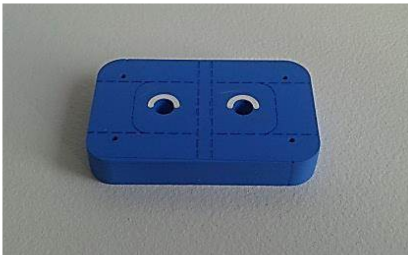
Figure 5.15: A set of two 3D coils of the same type on the same substrate after firing.
