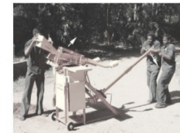
Automatic opening of the lid, while the operator fills the hopper
