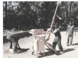
Starting the compression, while the operator fills the scoop
