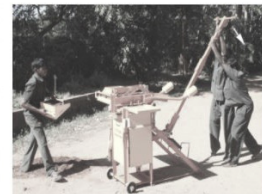
Pulling down the lever, while the operator supplies the mix
