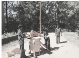
Opening the lid of the press by pulling the handle
