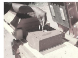
Checking the quality of compression with the pocket penetrometer (Only for the first block of every new mix)
