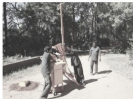
Sliding the hopper above the mould
