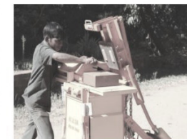
Sliding the hopper to push the block and to fill the mix into the mould
