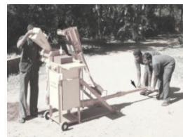
Ejection of the block, while the operator fills the hopper
