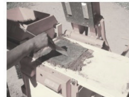
Scraping regularly the bottom plate with the scraper
