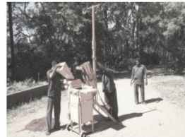
Feeding the press with the scoop into the hopper
