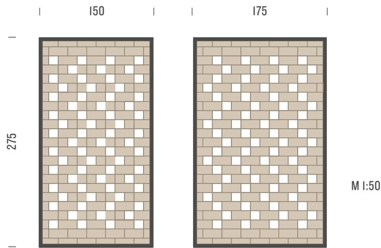
Fig. 5.10: Front view of the brick panels
