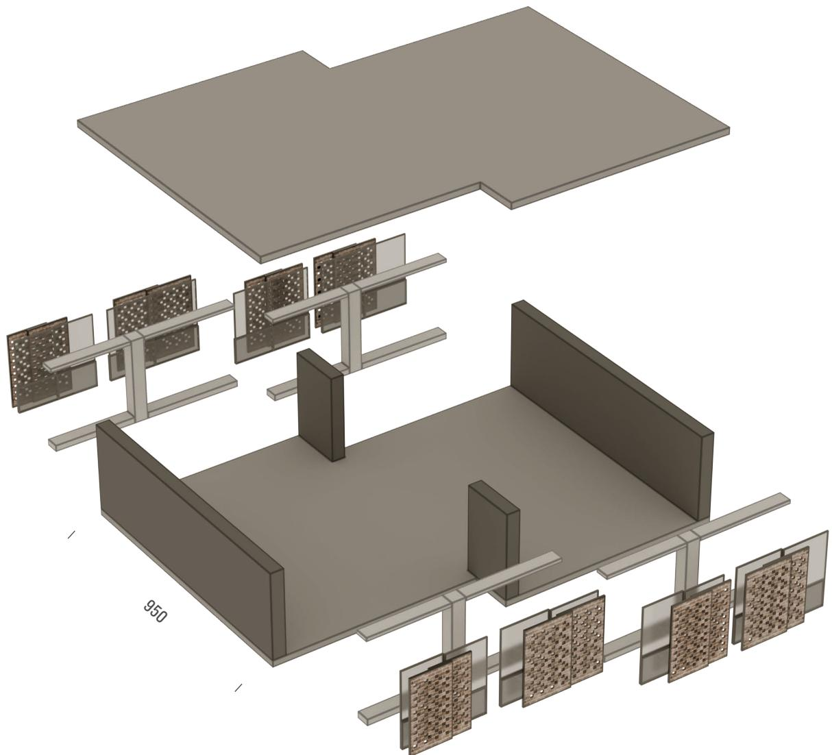
Fig. 5.29: The pre-fabricated parts of the *Home* project
