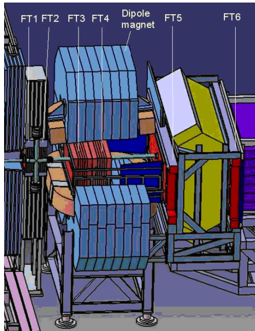
Figure 2.8: The forward spectrometer with indications for the six FTS planes is shown. Pictures taken from [8].
