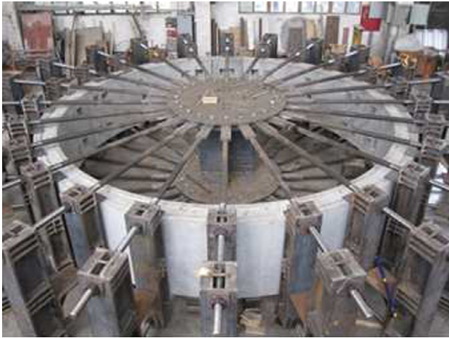
Fig. 1. Setup of the real-scale experiment of a segmented tunnel ring at Tongji University [1].
