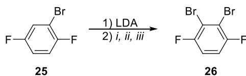
Scheme 31: Synthesis of 26 : 1) LDA (freshly prepared from DIPA and n -BuLi), THF, -80 °C; 2) - 80 °C, i ) F 2 Br 2 C ii ) Br 2 iii ) CBr 4 .
