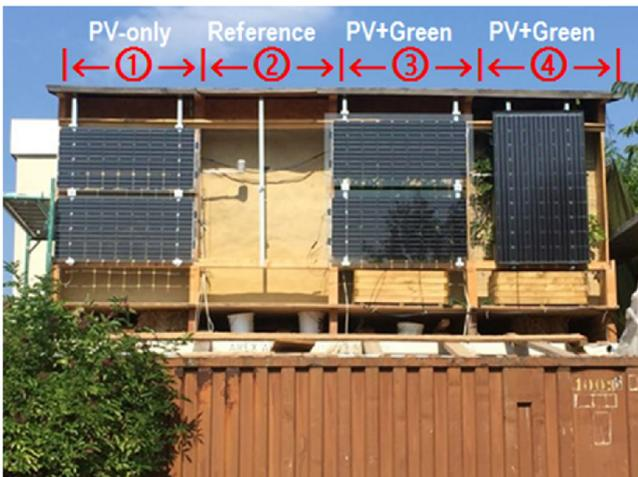
Fig. 6. Test area distribution. The differences between the components of each field's layout target the comparison of system-variations (fields – F#).
