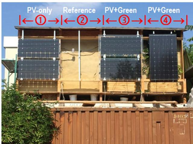
Fig. 4. Test area distribution. The differences between the components of each field’s layout target the comparison of system-variations (fields – F#).
