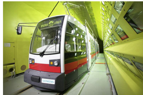
Fig. 8. Viennese Ultra Low Floor tram in the climatic wind tunnel, courtesy of “RTA Rail Tec Arsenal Fahrzeugversuchsanlage GmbH”.
