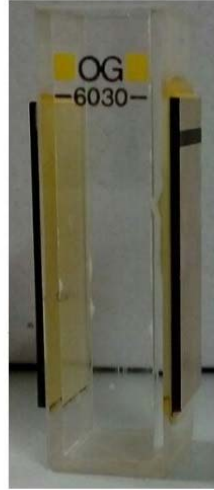
Figure 19) Cuvette 6030-OG- with two piezoelectric ceramics (PZT) glued to opposite sides of the cuvette
