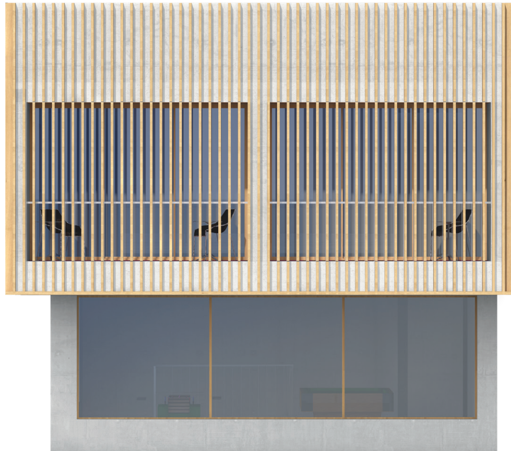
Fig. 4.3.4 Rotating fins for sun protection
