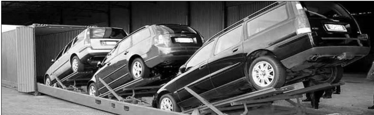
Abbildung 13: Spezialequipment Cronos Car Rack 3.7 (Cronos Group Limited 2014)
