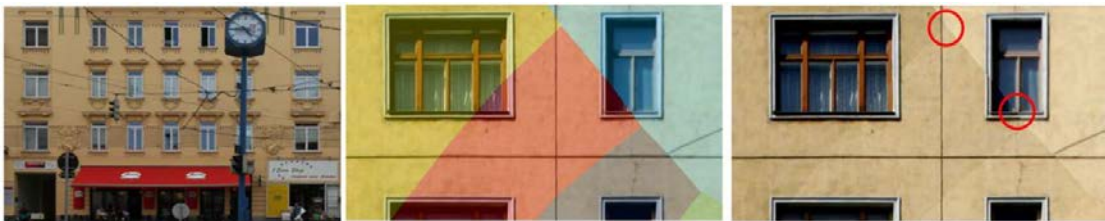
Figure 1.4: Texturing problems (screenshots created with a research prototype developed at the VRVis Research Center ): Occlusions (left) and the combination of multiple photos (indicated by colors, middle) lead to artifacts (right). The so-called stitching artifacts when using multiple photos are caused by different lighting conditions and camera settings in the individual photos.
