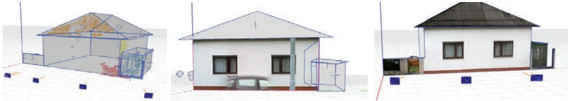
Figure 2.4: The reconstruction and modeling approach in the REPLICATE project (the screenshots have been created using the prototype developed in the project): Based on a computed photogrammetric data set consisting of oriented photos and a corresponding sparse, erroneous point cloud, a low-polygonal, CAD-ready geometric 3D model is created by exploiting detected planar segments, computed adjacency relations, extracted image edges and interactive snapping processes (left). The photos are first simply reprojected onto the geometry (middle). Through application of interactive brushing and/or texture synthesis methods, building surfaces free from stitching artifacts and occluders are created (right).
