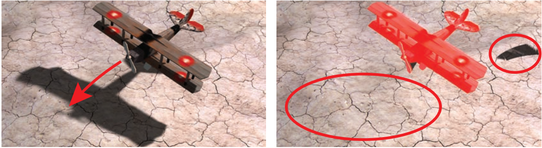
Figure 4.4: Shadows from a moving object. Left : Correctly shadowed scene of a moving toy airplane using PCSS. Right : Naive reprojection using depth comparison only recognizes that the shadow on the airplane needs to be updated, but does not indicate the need for a shadow recalculation in the regions marked with red ellipses.
