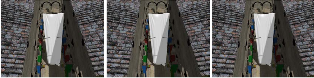
Figure 3.10: Visual Comparison using the complex Sponza Atrium scene: Left : Regular sampling with 289 shadow maps, acting as ground truth for our comparisons (2.5 FPS). Middle : Our method, 163 shadow maps (5 FPS). Right : Our method with only half the comparison render target size and a 3x3 PCF filtering requires only 14 shadow maps and is rendered at 40 FPS. See Figure 3.11 for difference images.
