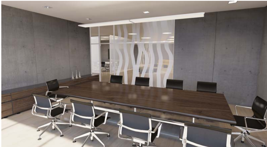
Figure 2.1: A recent screenshot of an office scenario designed and illuminated using the HILITE system [LTH + 13] with complex material system extensions [LTM + 14]. The actual light distribution is performed on the GPU using Shadow Mapping techniques. The accumulated light energy is iteratively accumulated in light-map textures. They are constantly updated in the visualization while the simulation is running, providing immediate feedback in interactive modeling sessions.
