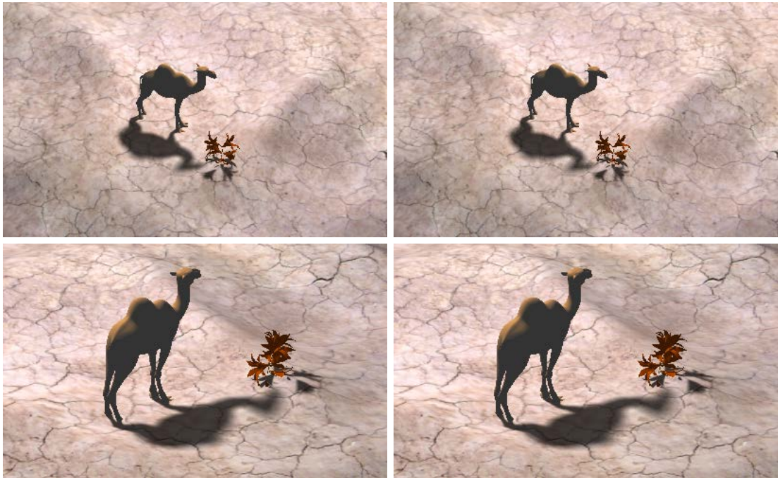
Figure 3.1: Our proposed method is capable of selecting and rendering a significantly reduced amount of shadow maps needed for a physically correct soft shadow solution using an adaptive light source subdivision. Top Left: Scene rendered from far with 289 fixed samples (10 FPS). Top Right: The same view point rendered with our method with only 25 samples (67 FPS). Bottom Left: The same scene, rendered from a closer view point with 289 fixed samples (10 FPS). Bottom Right: Our method reduces the number of needed samples to 105 (18 FPS).
