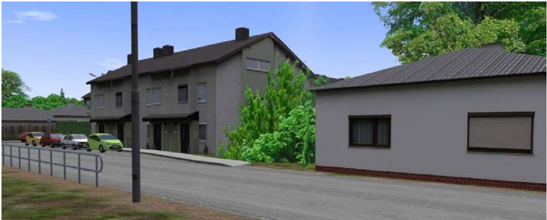
Figure 2.5: Buildings created with the prototypes developed in the REPLICATE project are used in a bus simulation software (OMSI 11 ). Notice the low-polygonal geometry, perfectly suited for real-time applications, and the textures generated from the photos: Even though they don't have any seams, they still suffer from shadowing artifacts, as the illumination contained in the photos has not been removed.
