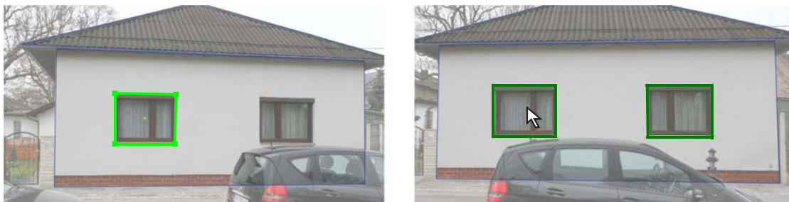
Figure 6.4: Multi-view sketching with suggestions. Left: The window is sketched in the first view and snapped to the image edges. In this case, no suitable planar point cloud segment is found, which is why the sketched 2D polygon cannot be projected to 3D space. Right: In a neighboring view, a search for similar polygons is performed in image space by using the histograms of the polygon edges of the source image. Two candidate polygons that resemble the same type of window are found. They are suggested to the user, and the left one is selected by a click.
