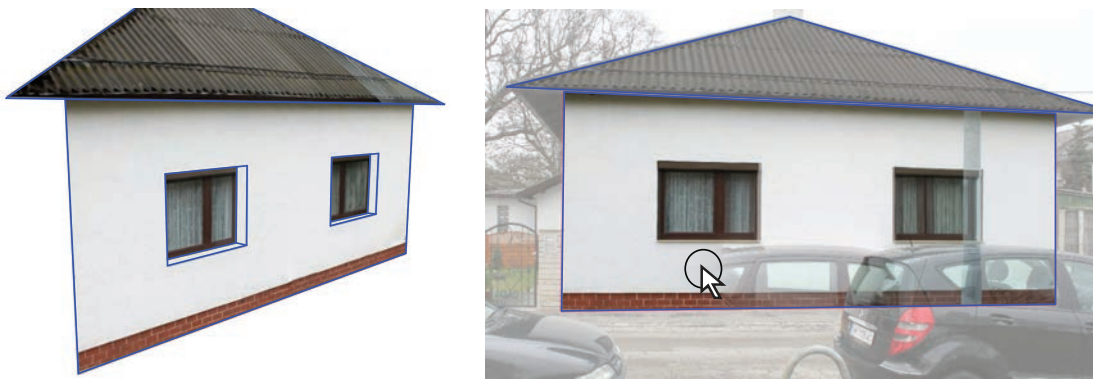
Figure 6.6: Left: By defining hierarchical relations, holes and side faces are automatically extracted. Right: Interactive removal of occluding objects from the texture by overlaying the photo semi-transparently using the shot view.
