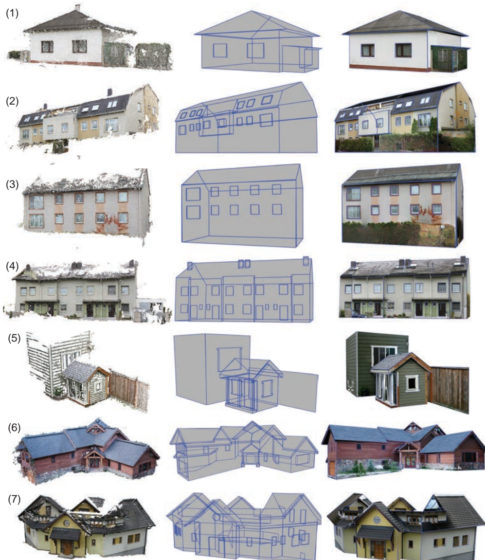
Figure 6.9: Textured 3D building models generated with our approach. Left: Photogrammetric point cloud. Middle: Geometric reconstruction including hierarchical definitions. Right: Final model with textures generated from multiple photos using the interactive occluder removal. Parts that are not depicted in the point cloud could be accurately reconstructed using the photos. The backsides of the houses 1-4 were modeled freely, as they were not accessible for the photographer. Buildings 6 and 7 were modeled using data sets with complete photo coverage from all sides, but required significantly more modeling time due to their complexity. For building 7, not enough photos were taken to model the roof completely. Modeling time including texture generation in minutes, from top to bottom: 5, 15, 10, 20, 15, 40, 45.
