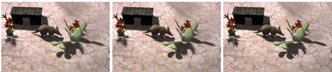
Figure 3.7: Visual Comparison of our approach. Left: Regular sampling with 289 shadow maps, acting as ground truth for our comparisons (8 FPS). Middle: Our method, 93 shadow maps (17 FPS). Right: PCSS soft shadow solution with visibility calculated from only a single shadow map (64/64 samples for blocker search/filtering step, 370 FPS). See Figure 3.8 for a visualization of the differences.
