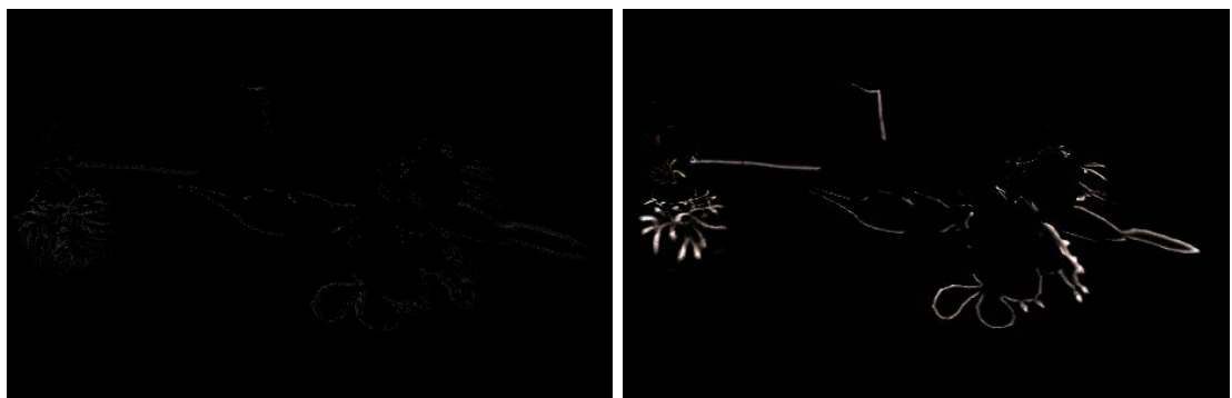
Figure 3.8: Left: Difference image between ground truth (Figure 3.7, Left) and our approach with 93 shadow maps (Figure 3.7, Middle), scaled by factor 5 for visualization purposes. Right: Difference image between ground truth (Figure 3.7, Left) and PCSS (Figure 3.7, Right), scaled by factor 5 for visualization purposes.
