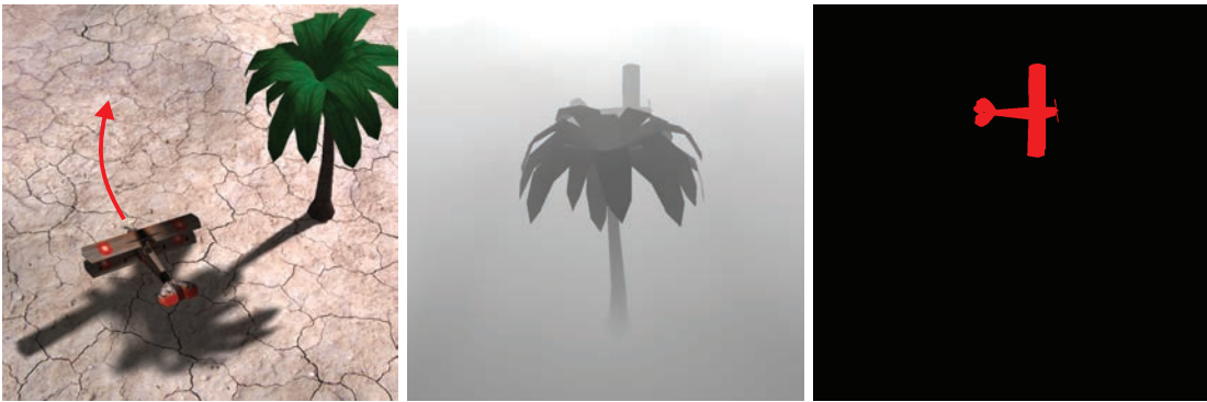
Figure 4.5: Shadow mapping extension for dynamic objects. Left : A scene with a static palm, casting a shadow onto the moving toy airplane. Middle : The depth map as known from the shadow mapping algorithm. Right : The corresponding Movement Map , indicating regions in which a moving object casts a shadow. Note that by rendering dynamic objects first, the parts of the airplane that are occluded by the palm can be stored as well. After the moving objects are stored, mipmaps are generated and used for an efficient lookup during the shadowing pass.
