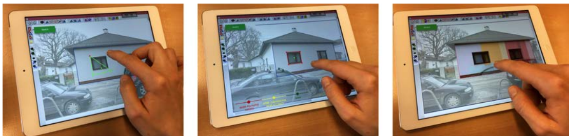
Figure 6.8: Evaluation of our proposed system on a touch-based device. Left: Coarse sketching of the polygon in the initial view. Middle: The polygon has been snapped to image edges and been reprojected to a neighboring image in the multi view sketching mode. The visual guidance feedback indicates that enough views have been used. Right: Interactive brushing.
