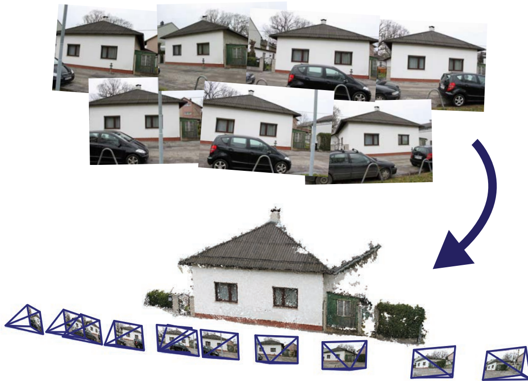
Figure 6.2: Photogrammetric Network (bottom), consisting of a 3D point cloud and photos (top), for which their relative positions and orientations have been computed. We refer to them as shots .
