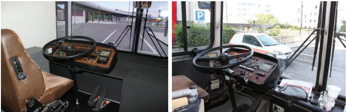
Figure 2.6: During the project, a hardware bus simulator (left) was built by our company partner ViewApp in order to increase both the immersion as well as the training effect. The bus simulation software including the reconstructed 3D buildings was coupled with the simulator hardware, perfectly replicating the behavior of driving a real bus through Vienna (right).
