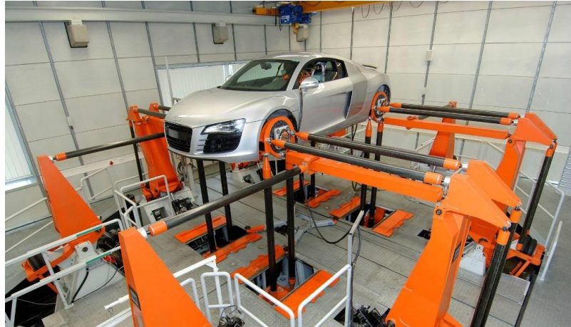
Fig. 16 Road simulator at AUDI AG (Hammer & Ehrich 2015)
