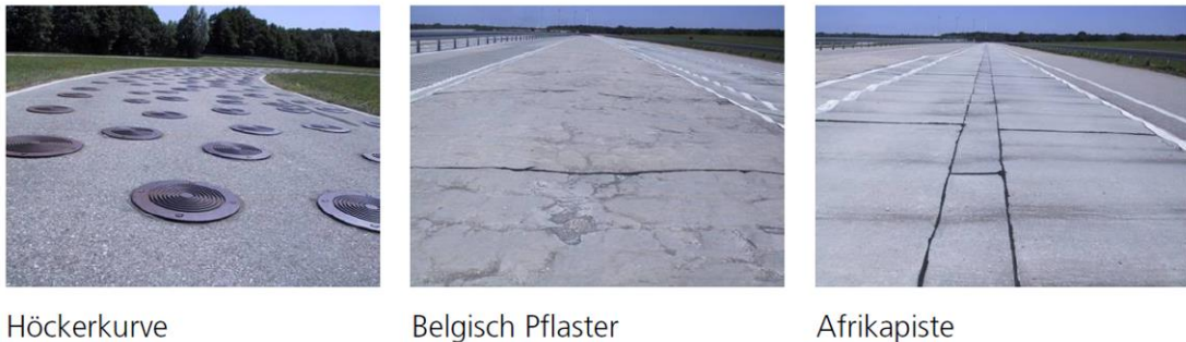
Fig. 14: Examples of different road sections on Audi's "Schlechtwegkurs" test track (Ungermann 2009)
