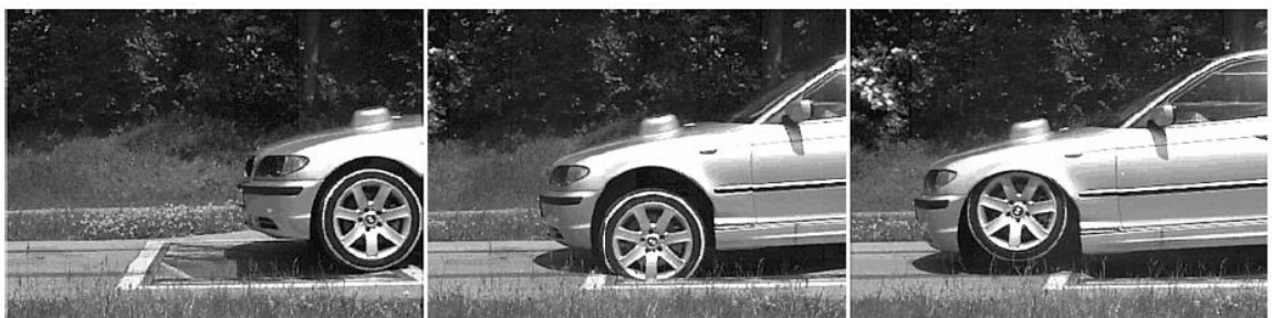
Fig. 13: Pothole misuse test (Weber 2009)
