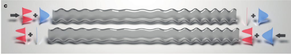
Figure 2.5: Two modes of a microwave passing a waveguide with modulated boundary conditions. Inserting from the left (right) side corresponds to encircling an EP (counter) clockwise. The waveguide acts as an asymmetric switch because the insertion direction affects which mode passes through. This figure is taken from [3].
