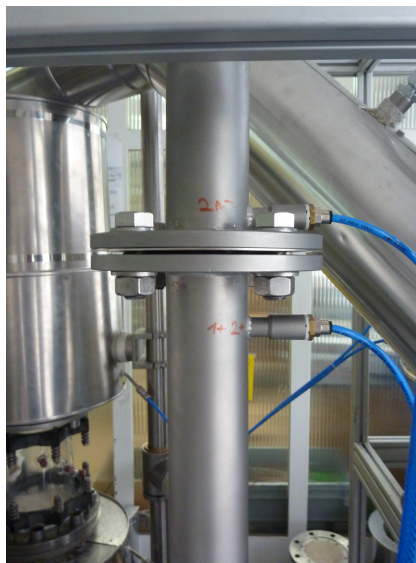
Figure 4.10: Flow measurement with orifice plate
