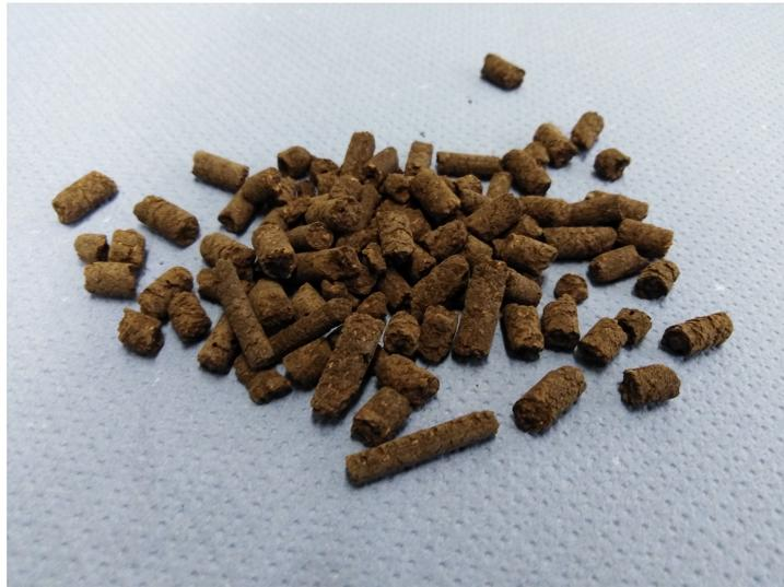
Figure 4.1: Olive pellet feedstock used for FBC
