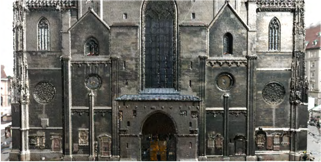
Figure 4.9: A huge laser scan of a cathedral (470M points) rendered by an out-of-core point renderer with Auto Splats. The renderer streams an amount of \sim 10\text{M} points to the GPU each frame.
