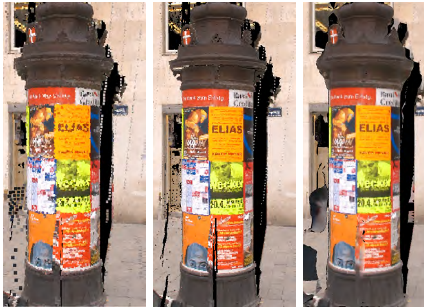
Figure 3.8: A scanned pillar point cloud rendered using screen-aligned box splats with heuristic density-based size [SZW09] (left), manually chosen optimal uniform splat size (center), and our screen-space triangulation method (right).
