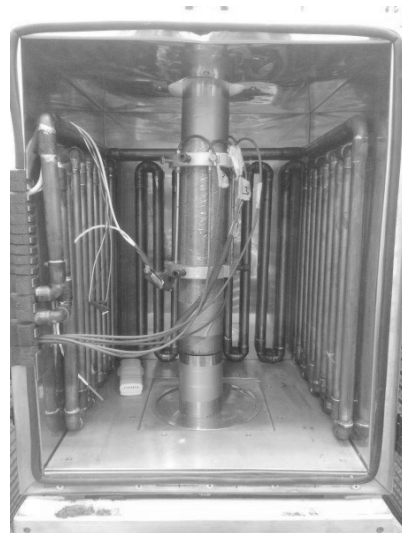
Figure 3. Test setup inside a temperature chamber containing two temperature sensors and copper pipes filled with conditioning fluid: two aluminum rings are attached to the concrete specimen, holding five displacement sensors; after [17].
