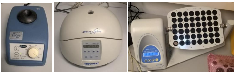
Figure 3.2.7: A) Stuart SA8 vortex mixer to mix the sample content and provide uniform attachment, B) Minispin Eppendorf centrifuge with a 12-place Fixed-angle rotor for 1.5–2.0 ml tubes (F-45-12-11) used to centrifuge the bacteria for washing purposes. Multiple washing was conducted during the sample preparation so as to eliminate the risk of non-specific binding. C) INCUBATOR&MIXER: multi-rotator Grant-bio PTR-60 to yield the binding between biological utilities and MPs.
