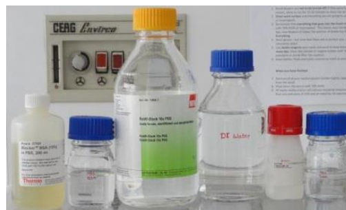
Figure 3.2.6: Chemical components required for preparation of washing and binding buffers: Blocker™ BSA (10%) in PBS, Roti®-Stock 10 × PBS, DI water and Tween® 20
