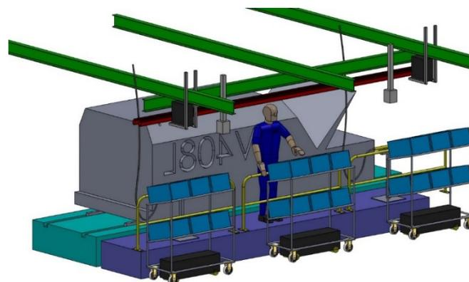
Figure 6.13: Design of overhead conveyor I
