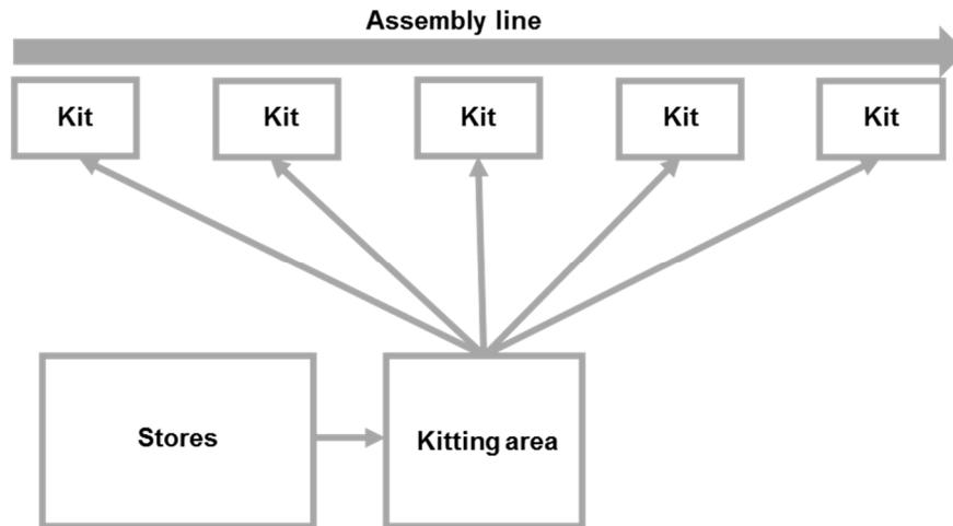
Figure 2.2: Kitting in a centralized picking area (Gajjar & Thakkar 2014: 895)
