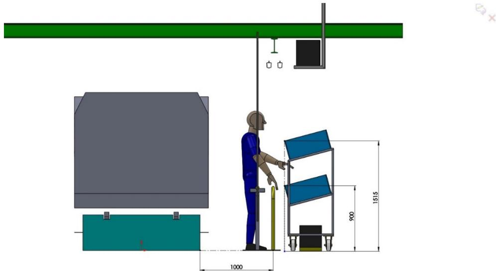
Figure 6.14: Design of overhead conveyor II
