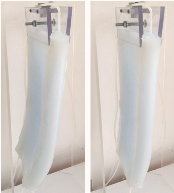
Δ69. Testing silicone by applying pressure into post-wax channel
