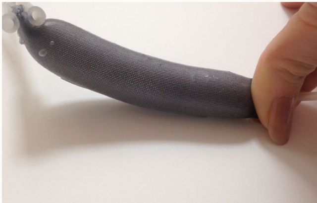
Δ71. Testing ecoflex silicon: creating a "textile pneumatic tube"
