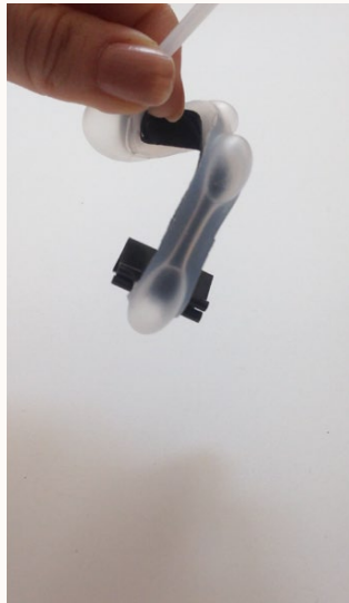
Δ72. Testing Ecoflex silicon : multilayered composite with integrated channel
