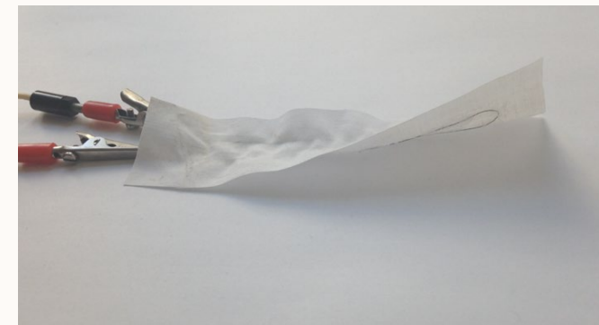
Δ70. Testing flexinol muscle wire mounted onto a piece of textile
