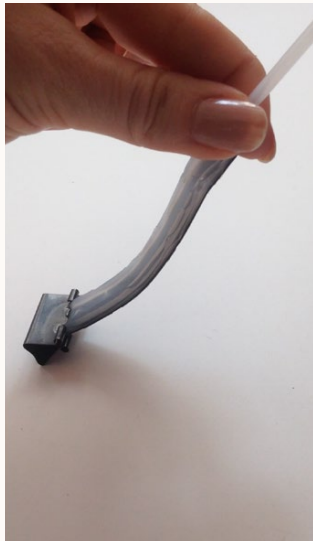
Δ72. Testing Ecoflex silicon : multilayered composite with integrated channel
