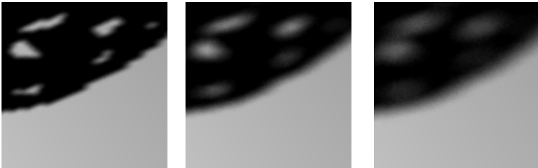
Figure 3.13: Side-by-side comparison of the same shadow silhouette rendered using different filter radii. The radius increases from left to right. The blocky artifacts resulting from the resampling error can be blurred with a filtering radius.
