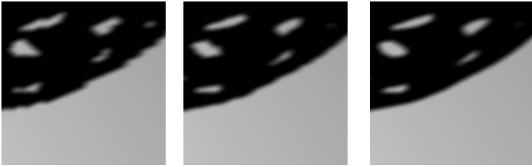
Figure 3.12: Side-by-side comparison of the same shadow silhouette rendered with different shadow map resolutions. The blocky artifacts tend to disappear with increasing shadow-map resolution.
