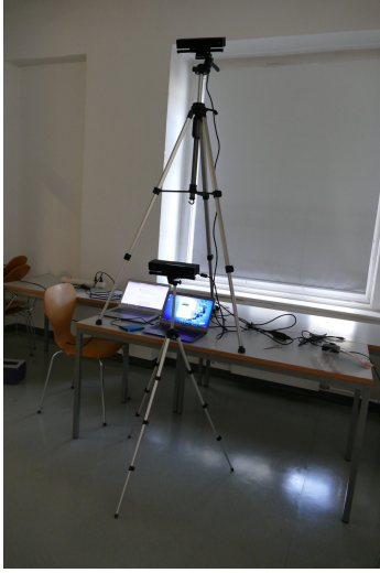
(a) Sensor setup: Two Kinect v2 placed in different heights using tripods.
