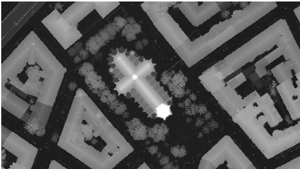
Figure 2.14: Example of DSM from the St. Othmar church in Vienna.
