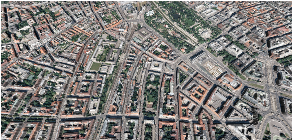
Figure 2.16: Textured surface created by interpolating raster data of DEM.
