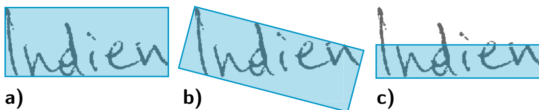
Figure 1.5: A bounding box which covers the whole CC a), the corresponding minimum area rectangle b) and the Profile Box proposed c).
