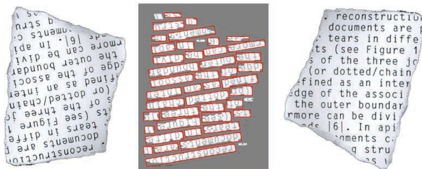
Figure 3.23: Document fragment; the word blobs of the document fragment gained using LPP and the corresponding minimum area rectangles; the corrected document fragment.
