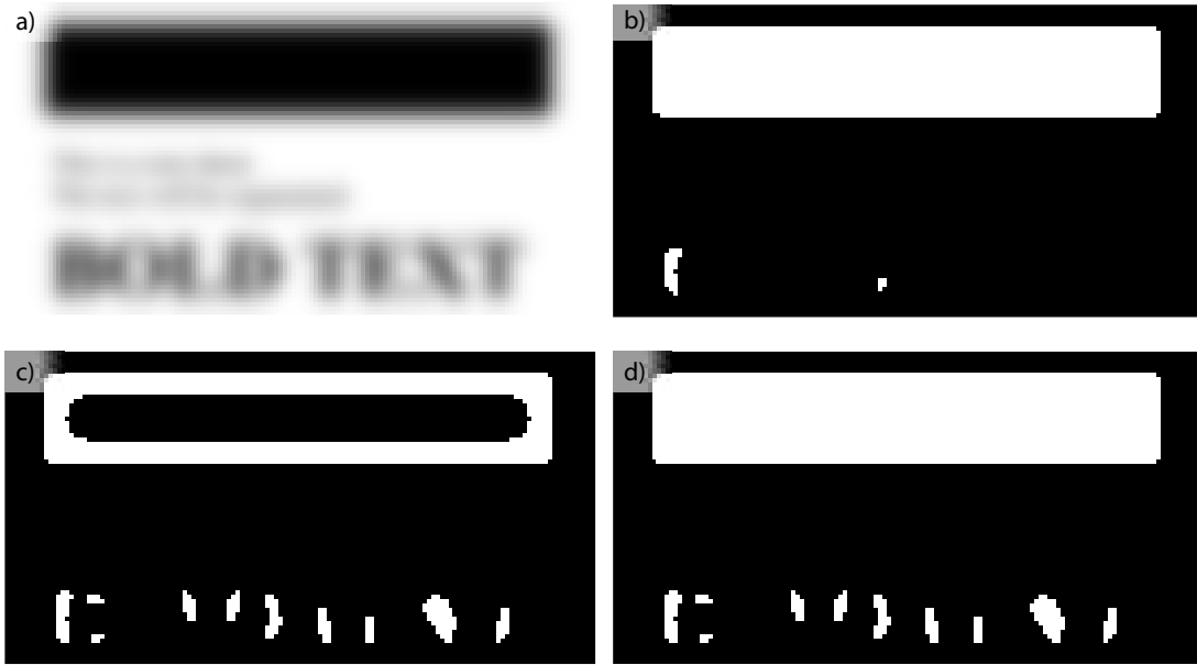
Figure 3.7: (a) current scale (b) parent image (c) current segmentation (d) scale space binarization
