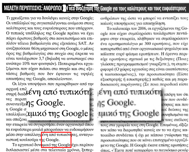
Figure 3.30: Resolution difference of the binarized images (left column) and the gray value images (right column) of DISEC 2013.
