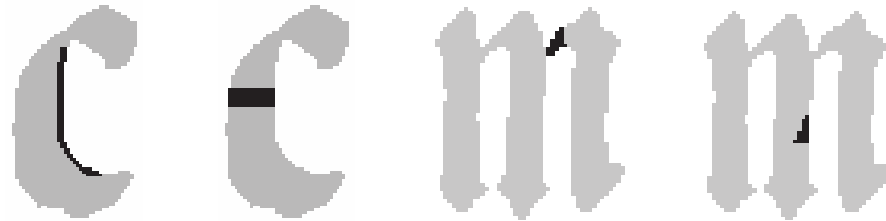
Figure 2.21: Two examples of characters with the same number of missing pixels (regarding each character) at different positions, courtesy of [126].
