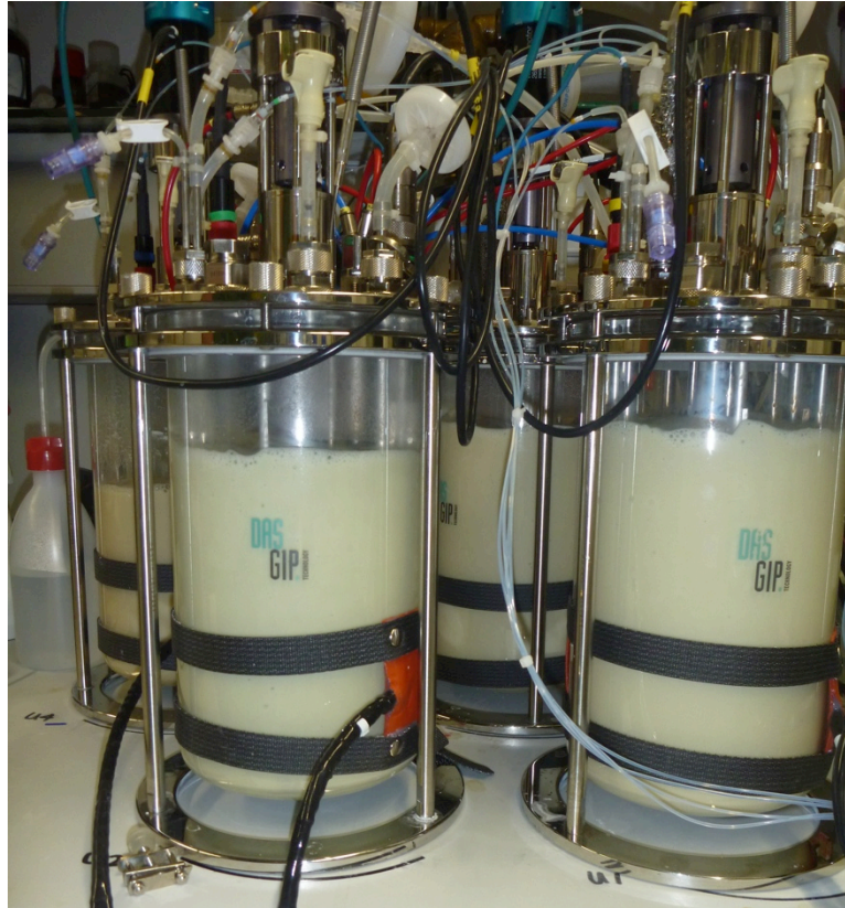
Figure 4: DASGIP-experiments as one-compartment system using 2.3 liter DASGIP-bioreactor. The DASGIP experiments had the advantage that you could run multiple reactors with different parameters such as DO, pH, T, simultaneously: Four one-compartment experiments were conducted at the same time with different DO level (5%, 25%, 70% and uncontrolled but above 25%).
