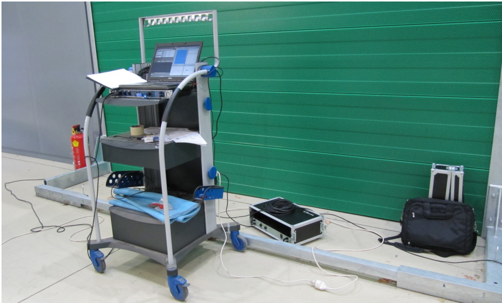
Figure 3.7: The computer, audio interface and amplifier that were used for the measurements
