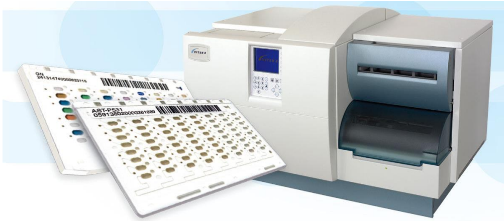
Fig. 1.1.5: The Vitek 2 automated ID/AST instrument from BioMérieux. The disposable reagent cards have 64 wells that each contain an individual test substrate. Substrates measure various metabolic activities such as acidification, alkalinization, enzyme hydrolysis, and growth in the presence of inhibitory substances. An optically clear film present on both sides of the card allows for optical read out using different wavelengths in the visible spectrum to measure either turbidity or colored products of substrate metabolism. Picture taken from www.biomerieuxconnection.com .
