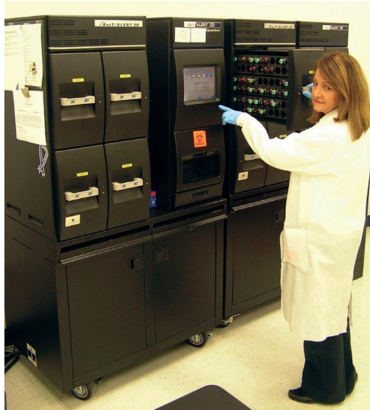
Fig. 1.1.4: The BacT/ALERT® 3D instrument from BioMérieux is a state-of-the-art, automated microbial culture and detection system. The system is based on the detection of CO 2 released by actively proliferating bacteria into the liquid media. CO 2 lowers the pH in the growth media, which in turn produces a color change in a sensor in the vial, detected by a reflectometric unit in the instrument. Picture taken www.biomerieuxconnection.com .
