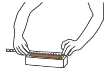
7 if soil is completely dry measure how much soil has shrunk
