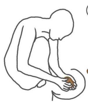
2 first do a "ball falling test" and form balls of clay with a diameter of 5 cm
