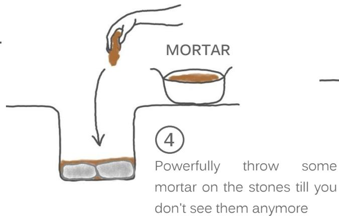
attention prepare clay mortar two days before beginning piling foundation (as shown on next page)
