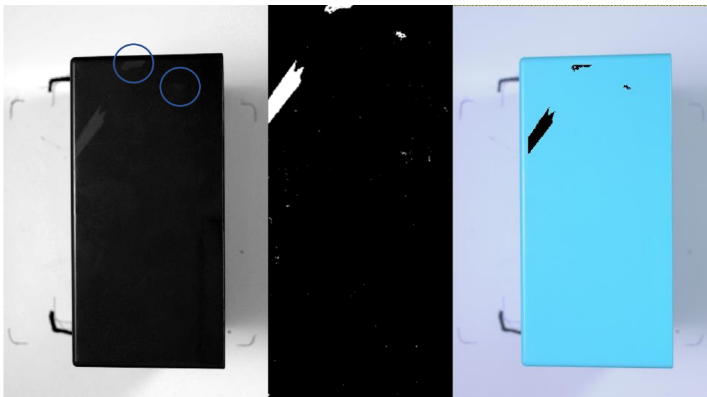
Figure 4.30: Cyan sample 1: left: red layer of the defected cyan part (original image); middle: dichotomized image of the detected defects; right: image-stack of the size-relevant defects and the original RGB photograph
