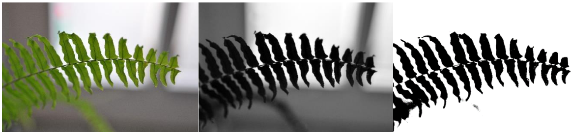
Figure 2.11: Binary image segmentation using a threshold; left: original image; middle: blue layer; right: segmented image
