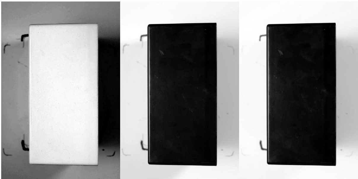
Figure 4.13: Left: red layer of red sample part; middle: green layer of red sample part; right: blue layer of red sample part
