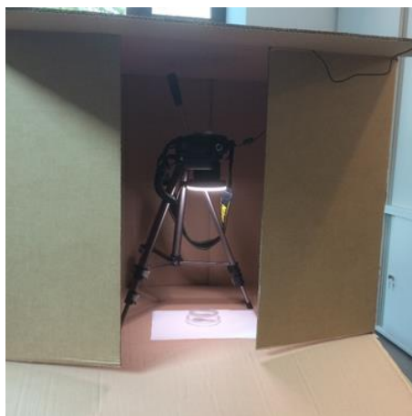
Figure 4.1: Experimental setup for defect detection of transparent circular shaped lids
